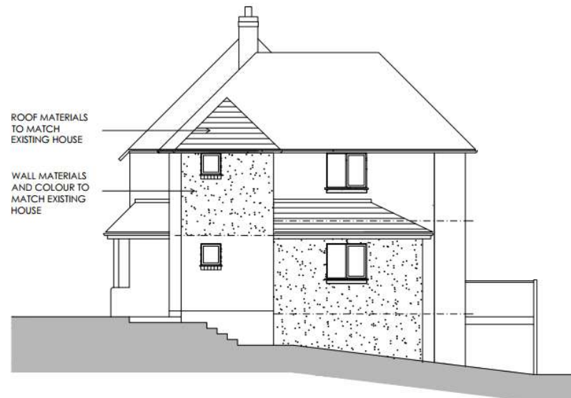
SIDE / EAST ELEVATION
