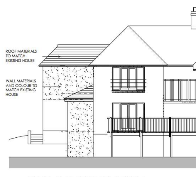
REAR / NORTH ELEVATION
